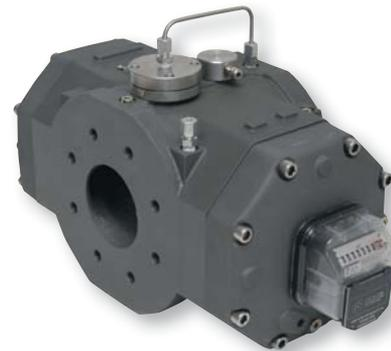
Meter with external bypass option. In the unlikely event of a flow blockage, gas supply is guaranteed. An electrical contact can be wired to activate an alarm.
