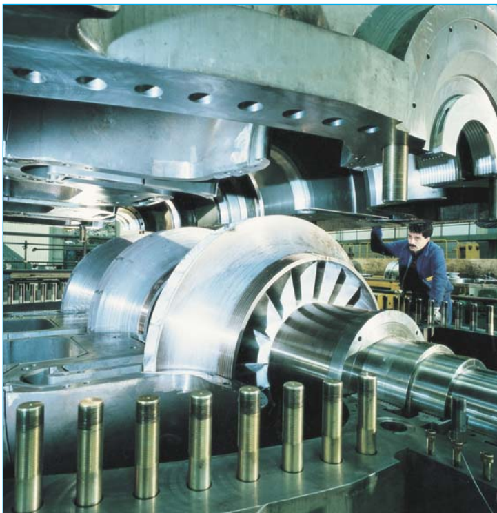
Large horizontally split compressor
